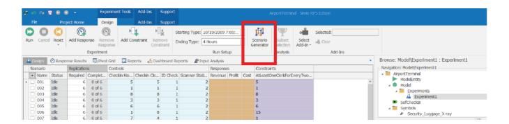
With Scenario Generator, users are given an efficient way to create a full factorial Experiment for a model based on the number of controls and the subsequent levels of each control.
