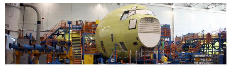
The first six tasks in Work Cell 3 require an overhead crane. The crane must be available to be used by Work Cell 3 before the first task (Operator obtains crane & attach) begins and it must stay at Work Cell 3 until the sixth task (Install Tack Fastener) is finished. A second production line would require coordination of this overhead crane because it would need to be shared between Work Cell 3 in both lines.
